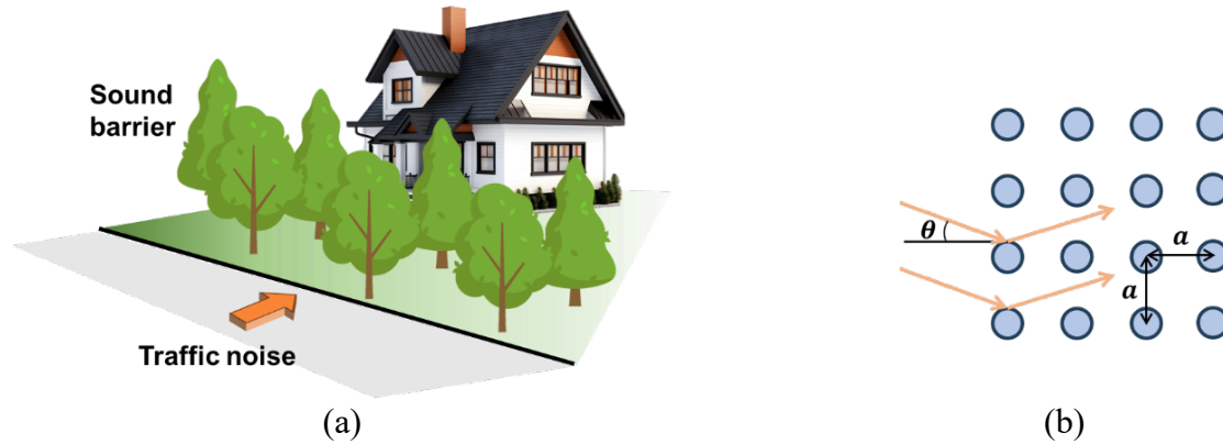
Fig 1. (a) Tree sound barriers, and (b) schematic of sonic crystal alignment.
