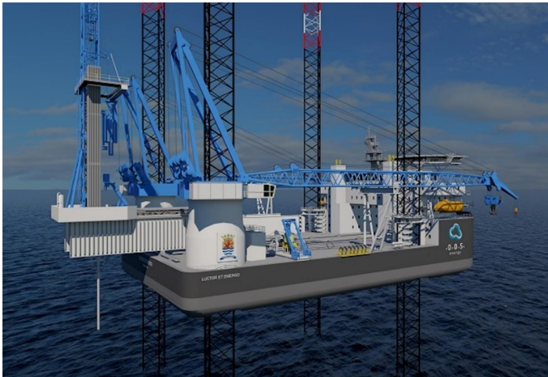
Fig. 3. The OOS drilling-rig-based intervention platform.
