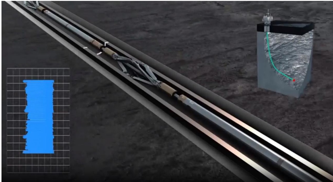
Fig. 19. Baker Highes Certia technology for free pipe depth detection.
