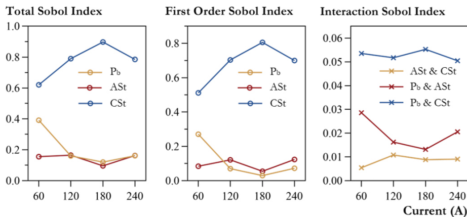
Figure 10. Different order of Sobol indices along with back pressure and Stoichiometry at different current densities.
